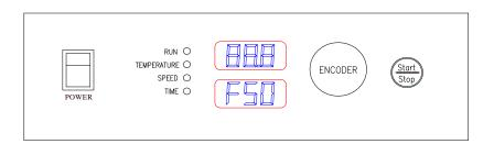
• Press and hold encoder knob for more than 2 seconds. Temperature signal light blinks. With rotating encoder clockwise (+) or counter-clockwise (-), set temperature to desired value:
